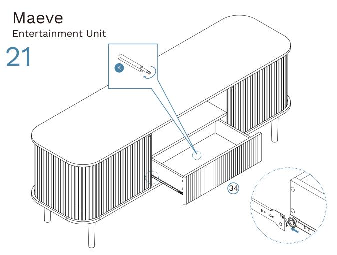
Insert the assembled drawers into the corresponding compartments as shown. Ensure the drawers slide easily along the rails. If the door is not catching or sitting flush, twist the end of the cover (K) until it catches on the seal (L).
